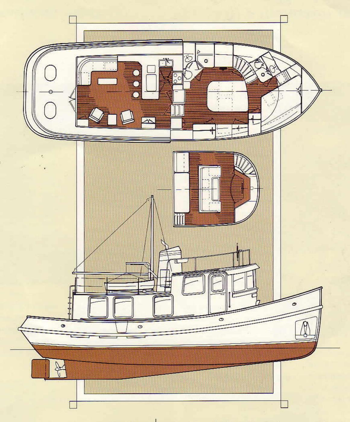
LOA ~ 48' 10" LOW ~ 45' Beam ~ 16'-8" Draft ~ 4'-10" Displacement ~ 58,000 lbs Ballast ~ 8,500 lbs. Engine ~ 250 hp Cummins
